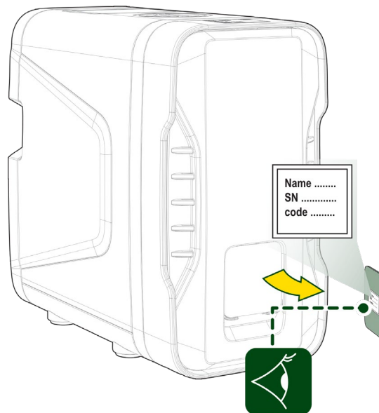
Fig. 4 Metal plate - Location of product information label
